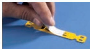
3. Seal the carrier by placing a finger on the film and pushing forward, thus rolling over the film and rolling off the silicon liner.
